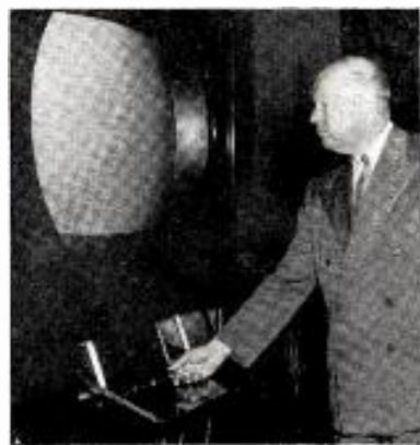
REFLECTING the growth of the television industry is this 30-inch direct view screen television receiver (picture is 536 sq. in.) claimed by DuMont to be the world's largest. Dr. Allen B. DuMont, head of Allen B. DuMont Labs and DuMont Television Network, adjusts a control dial on the "Club 30" set which he introduced at the first national convention of DuMont distributors held July 6-7 at the Hotel Pierre in New York [TELECASTING, July 10].
